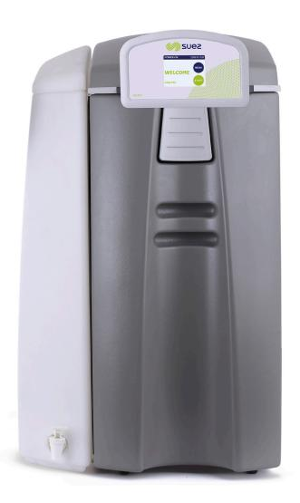
The Select Analyst is a compact unit ideal for laboratory use, delivering a steady supply of >  $1M\Omega$ .cm pure water for laboratory tasks using carbon pre-treatment, reverse osmosis and deionisation.
